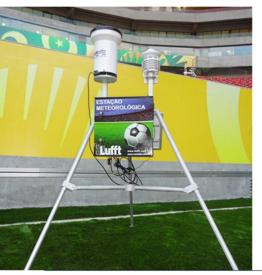
The weather stations measure temperature, relative humidity, air pressure and global radiation. In addition, an external rain gauge can be added to measure rainfall. Thanks to the energy-saving mode, the WS301-UMB weather sensor can be used mobile and solar-powered. The stations were located behind the goals. That's why they were visible on TV and in the press, as you can see in the pictures of the Confederations Cup match for third place (Uruguay - Italy) to the left.
